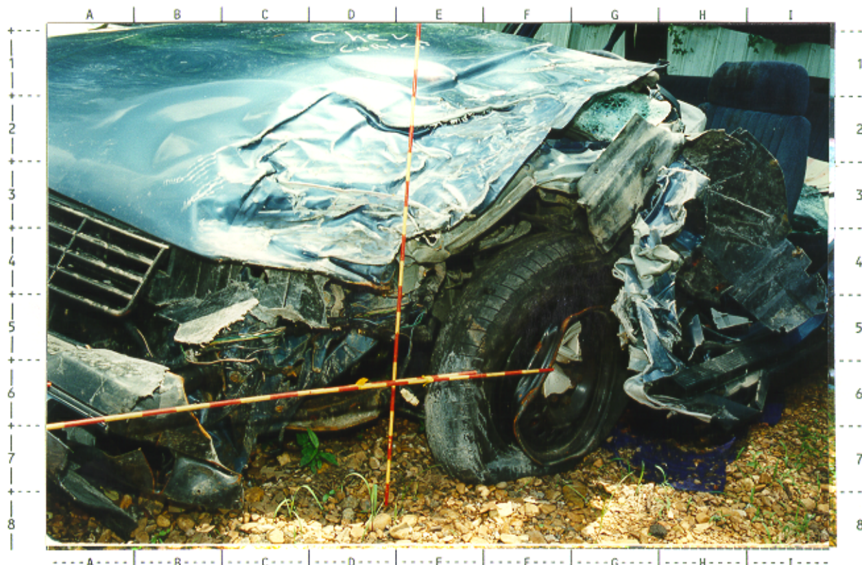
# 38 -- Close-up front left (45 degree angle) view of 1991 Chevrolet Corsica's damage to left front tire and rim
